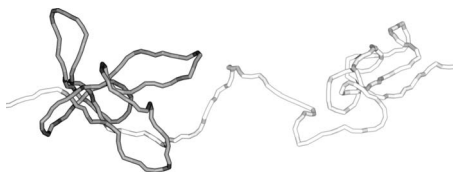
FIG. 2. Calculation of the knot size. After eliminating all of the trivial crossings, the entire right coiled part of the chain conformation was disentangled. The part of the chain contour which was determined by our algorithm as the knot is marked by the dark tone.
